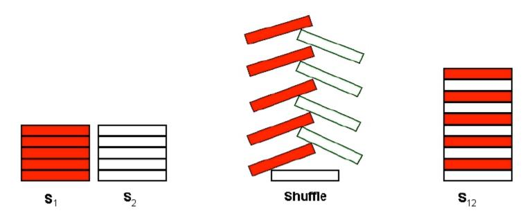
The single resultant stack,  $S_{12}$ , contains  $2^*C$  chips. The bottommost chip of  $S_{12}$  is the bottommost chip from  $S_2$ . On top of that chip, is the bottommost chip from  $S_1$ . The interleaving process continues taking the  $2_{nd}$  chip from the bottom of  $S_2$  and placing that on  $S_{12}$ , followed by the  $2_{nd}$  chip from the bottom of  $S_1$  and so on until the topmost chip from  $S_1$  is placed on top of  $S_{12}$ .
